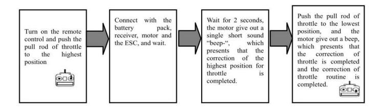
• The normal startup procedure of the ESC is as follows:
