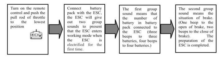
Remark: if the motor suddenly stops when your model airplane are flying, you shall immediately push the pull rod of throttle to the lowest position and then push to the high position. Then the motor will restart. You shall land the model airplane immediately with throttle controlled with a lower position.
